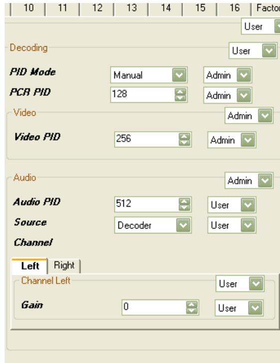
Figure 5-12: Receiver Video and Audio Decoding Settings
