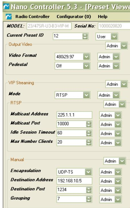
Figure 5-9: Receiver Factory, Output Video and VIP Streaming
