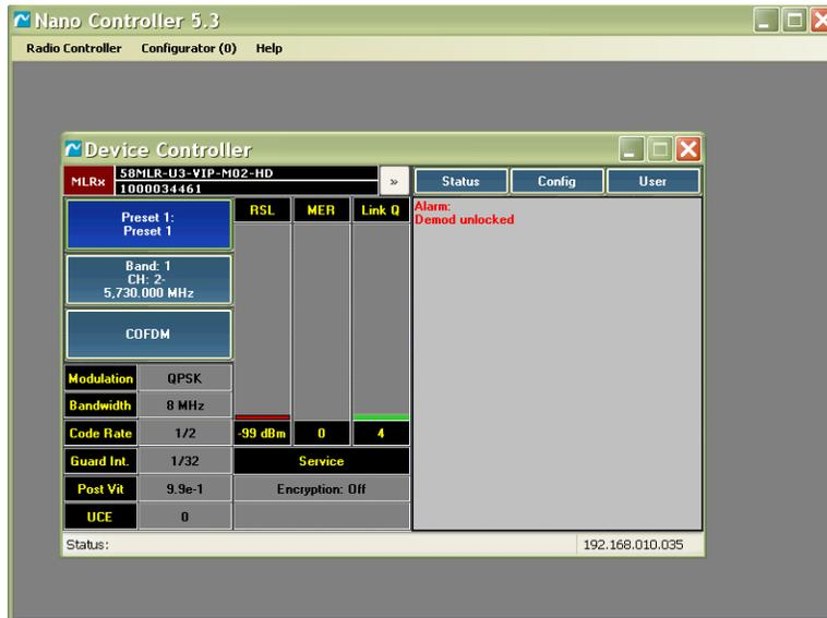
Figure 4-1: Receive Device Controller window
